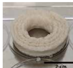
Whole scaffold of a fiber-based additive manufactured silk used to mimic an intervertebral disc. © Courtesy of Benjamin Gantenbein
